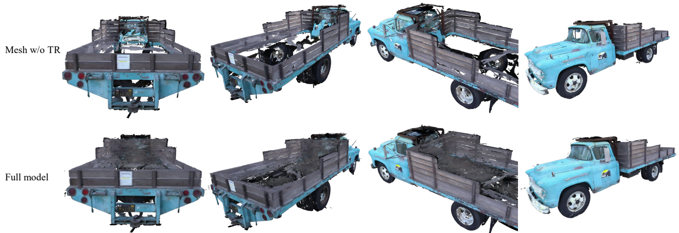
Fig. 7: Effect of the Target Replenishment (TR) Module. The first line shows the mesh generated solely using Target Gaussian Segmentation. The second line displays the mesh produced by our complete model, including the Target Replenishment module. The significant loss of information in the input views results in numerous missing parts in the mesh. However, experimental results show that TR can fill in the missing parts while keeping the visible parts unchanged.
